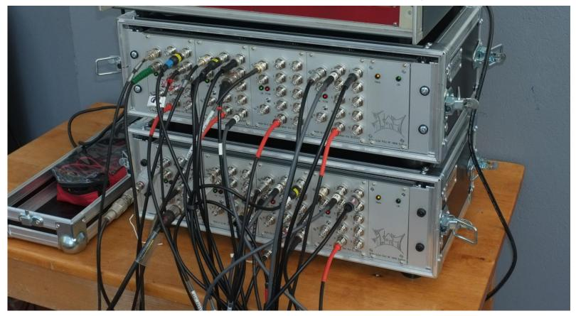
Antenna signal distribution Racks. Each 19 inch rack houses 4 active Antenna Multiplexers /Bias Tee – one antenna Input > 12 user out, and a linear power supply. Multiple antennas are simultaneously available to all users.
